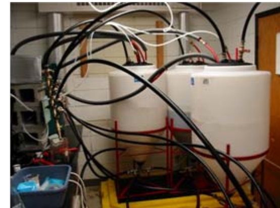
Figure 3: Greentech's early 60 gallon scale biodiesel manufacturing prototype. In Winooski, we use reactors that are up to 10 times larger.
